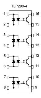
1,3,5,7 :ANODE, CATHODE 2,4,6,8 :CATHODE, ANODE
