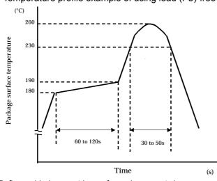
This profile is based on the device's maximum heat resistance guaranteed value.
