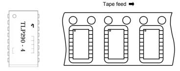
Figure 1 Device Orientation
